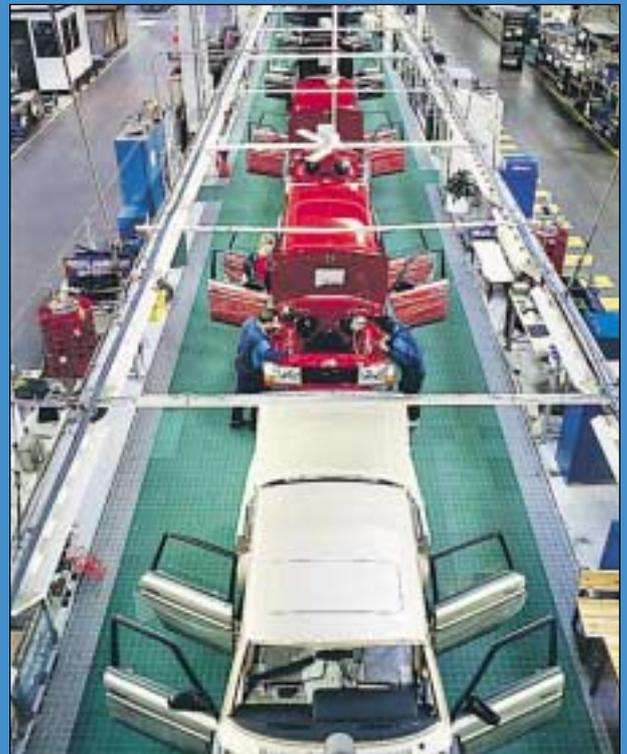
In 1913, Henry Ford revolutionized the production process of a car by pioneering mass-production manufacturing, a production system in which a conveyor belt brings each car to the workers, and each individual worker performs a single task along the production line. Even today, cars are built using this system, as shown in this photo of workers along a computerized automobile assembly line.
